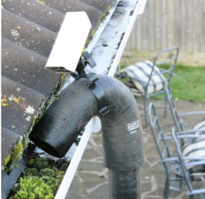
The Gutter Vac operates solely from the ground using special cameras to view the roof and gutters
